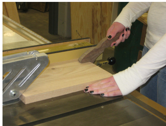
Proper use of saw: comfortable Position & stance, Out of line of blade
